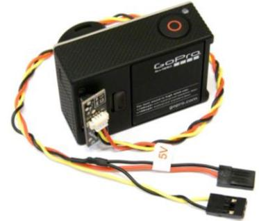
You can charge GoPro camera by connecting **5V** cable (black-red) to RC receiver other 5V source.
