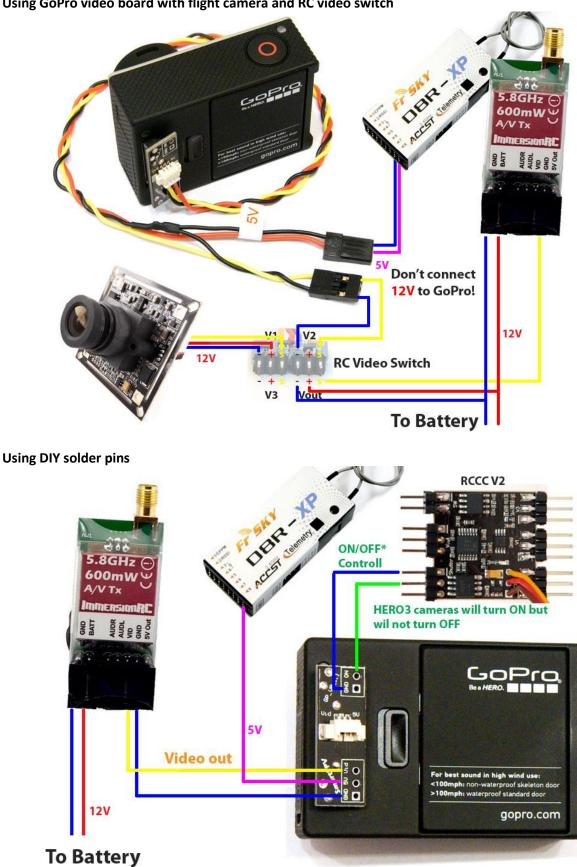
Using GoPro video board with flight camera and RC video switch
