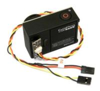
You can charge GoPro camera by connecting **5V** cable (glack-red) to RC receiver other 5V source.
