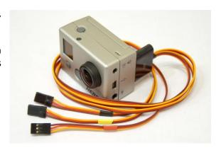
You can use video out from camera, charge camera from RC receiver and record HD video at same time.
